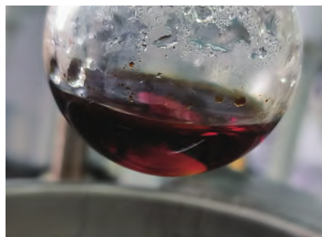
Fig 6 Phenolic resin glue prepared by students
